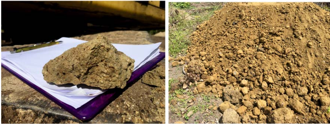
Figure 7: Dense sandy layer on left picture. Usual GU1 appearance for right one
